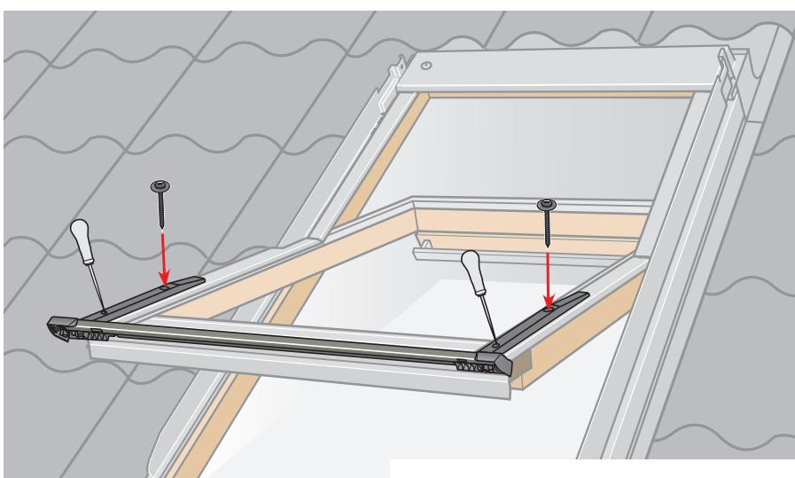
**ENGLISH:** Fit storm brackets and bottom cover temporarily with screws in the upper holes. Make a mark with bradawl through the lower holes.
