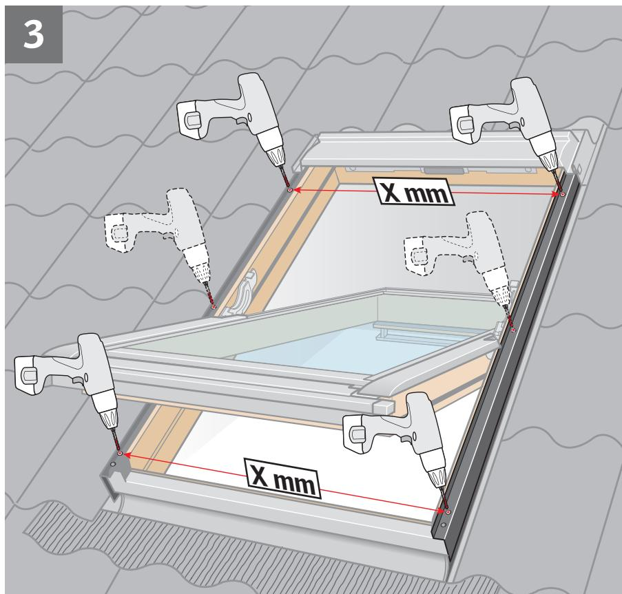
**ENGLISH:** Drill a hole through the marks in the side frame covers **a**. To ensure that the roller shutter runs efficiently, the distance ( $X \text{ mm}$ ) between the side frame covers at top and bottom must be exactly the same.
